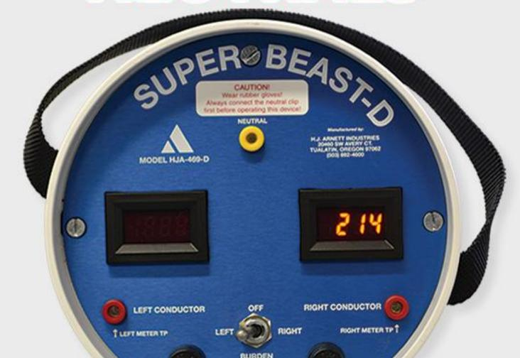
Test: Flip Switch Left Left Meter: Blank Reading, Nothing Shown Right Meter: Increases Significantly, +50V **Reading: Fully Open Neutral**
