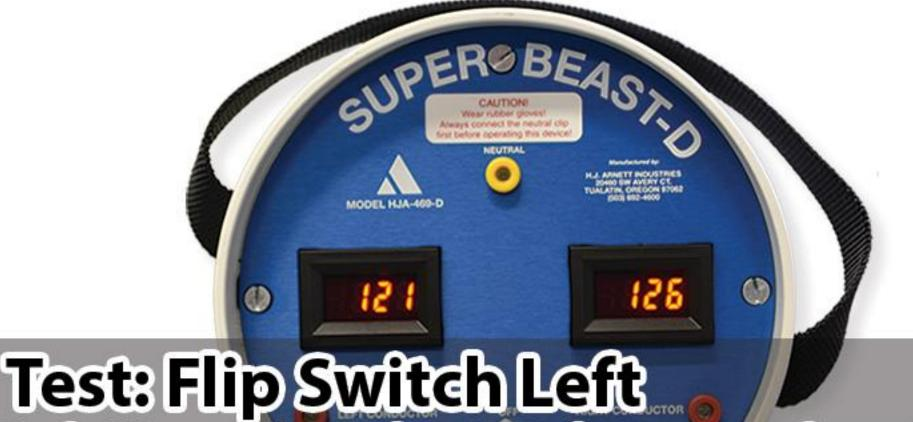
Left Meter: Less than 5% drop = good conductor Right Meter: Remains the same / ±1V Reading: Good Left Conductor
