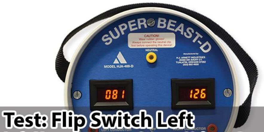
Left Meter: 5-7% or Greater Voltage Drop Right Meter: Remains the same/±1V
