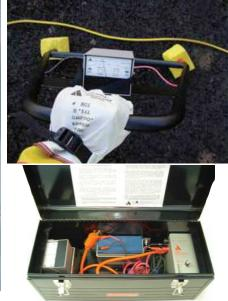
Use the A-Frame to easily locate faults over concrete simply by placing sponges wet with salt water on the end of each probe.
