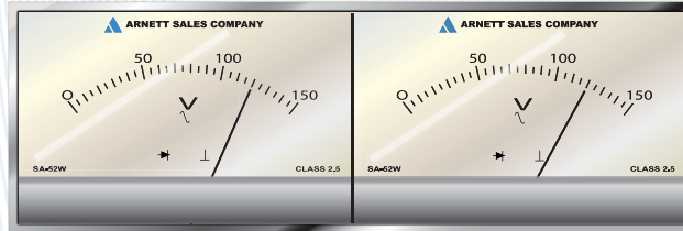
Left meter reads 120V, so left conductor is OK.
