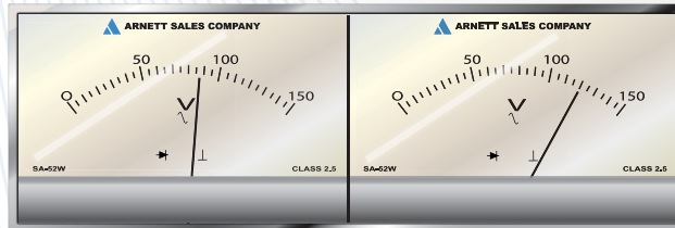
Only left meter drops, so left conductor is partially open. If left meter drops to zero, left conductor is fully open.
